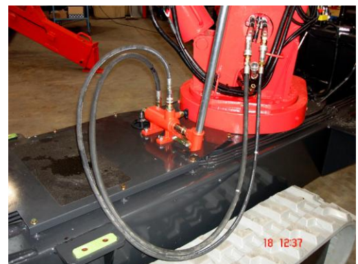
Illustration 5 showing crane ready for emergency winching
