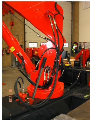
Illustration 3 showing crane ready for emergency telescoping Note the telescoping adaptor (D) fitted to the line
